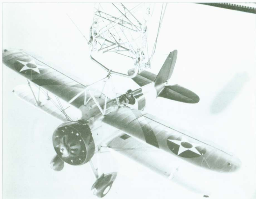
A Sparrowhawk bi-plane hooked onto its "arrester" and suspended from the retractable trapeze. The tiny shadow of the airship, at center right, suggests the Macon's height during this intricate manoeuver. NPS photograph.
